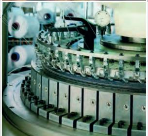
Example of application: Functional check of a circular knitting machine during running operation.
